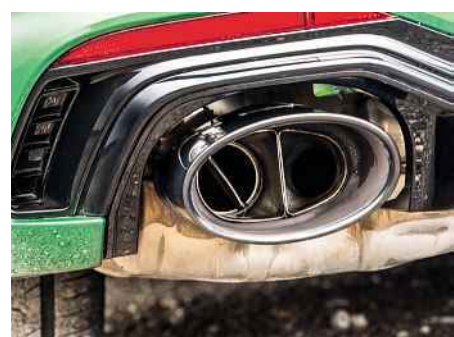
Above: exhaust valve beefs up the sound of the turbo'd V6 when the car is in its sportier modes. Left: cabin quality is ahead of that of the RS5's rivals
