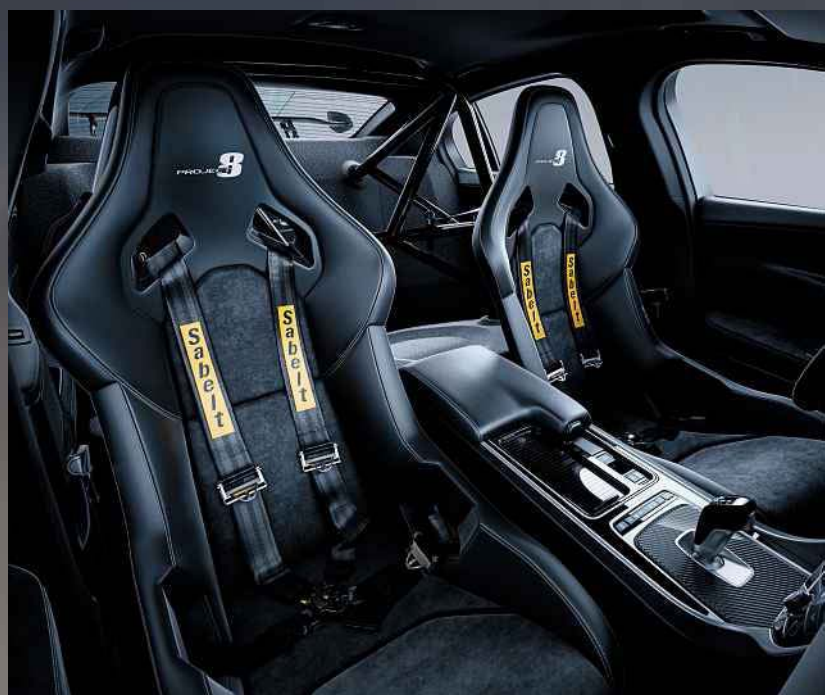
Above: Track Pack sees a half roll-cage fitted for the full touring-car vibe. Left: wider arches house huge 305-section tyres at the rear – handy when you're putting down nearly 600bhp
