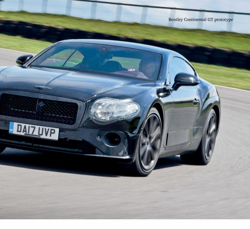
a much leaner, sportier aesthetic. The weight distribution is also significantly improved, with a 52:48 split front to rear (the old GT was 56:42), and the car is around 100kg lighter. Okay, so that's still over two tonnes, but then Bentley isn't skimping on the luxury aspect.
