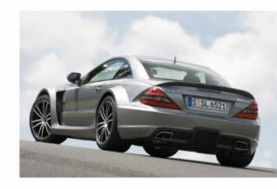
Above and main: with a 493kW twin-turbo 6.0-litre V12, the SL65 Black Series remains the most powerful Mercedes product fitted with an internal combustion engine.
