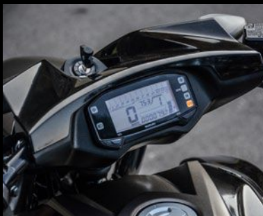
The Intruder 150 uses the same all-digital instrument cluster as the Gixxer. Other highlight features of the baby Intruder include automatic headlamps, LED tail lamps and front & rear disc brakes. The Intruder 150 also comes with ABS as standard.
