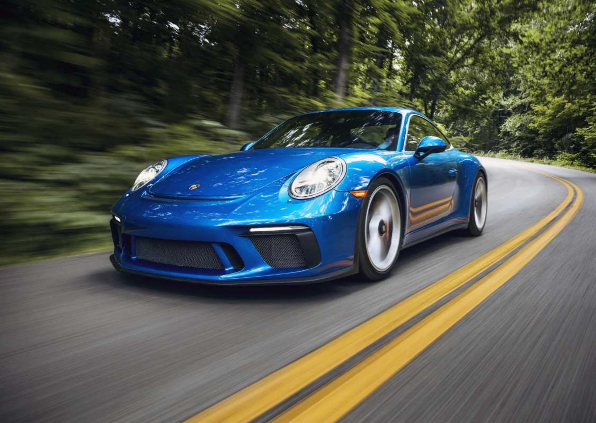
Dive down an exit ramp into some Appalachian foothills, though, and you'll be happier still. Your fingertips tingle with feedback from the front 245/35ZR-20 Michelin Pilot Sport Cup 2s, which generate enormous grip despite being the narrowest in the test. It helps that they're supporting just 40.1 percent of the GT3's weight, which, at 3303 pounds, is more than 400 pounds lighter than either of the other cars.
