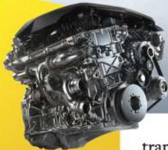
The B48 four-cylinder and B58 six-cylinder engines in the new 3 are members of BMW's modular engine family, which is based around 500-cc cylinders.
