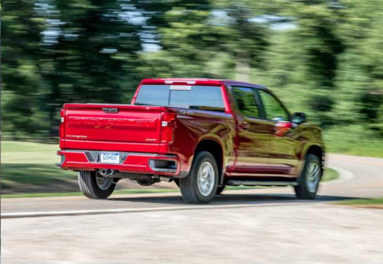
hundred pounds for some models, and the Silverado's new bed is constructed in three pieces, which allows the wheel wells to be stamped differently, increasing cargo volume to 63 cubic feet in short-bed models. Compare that with the Ram 1500's bed at 54 cubic feet and the F-150's at 53 cubic feet, and things are starting to look good for Chevy's usurper.
