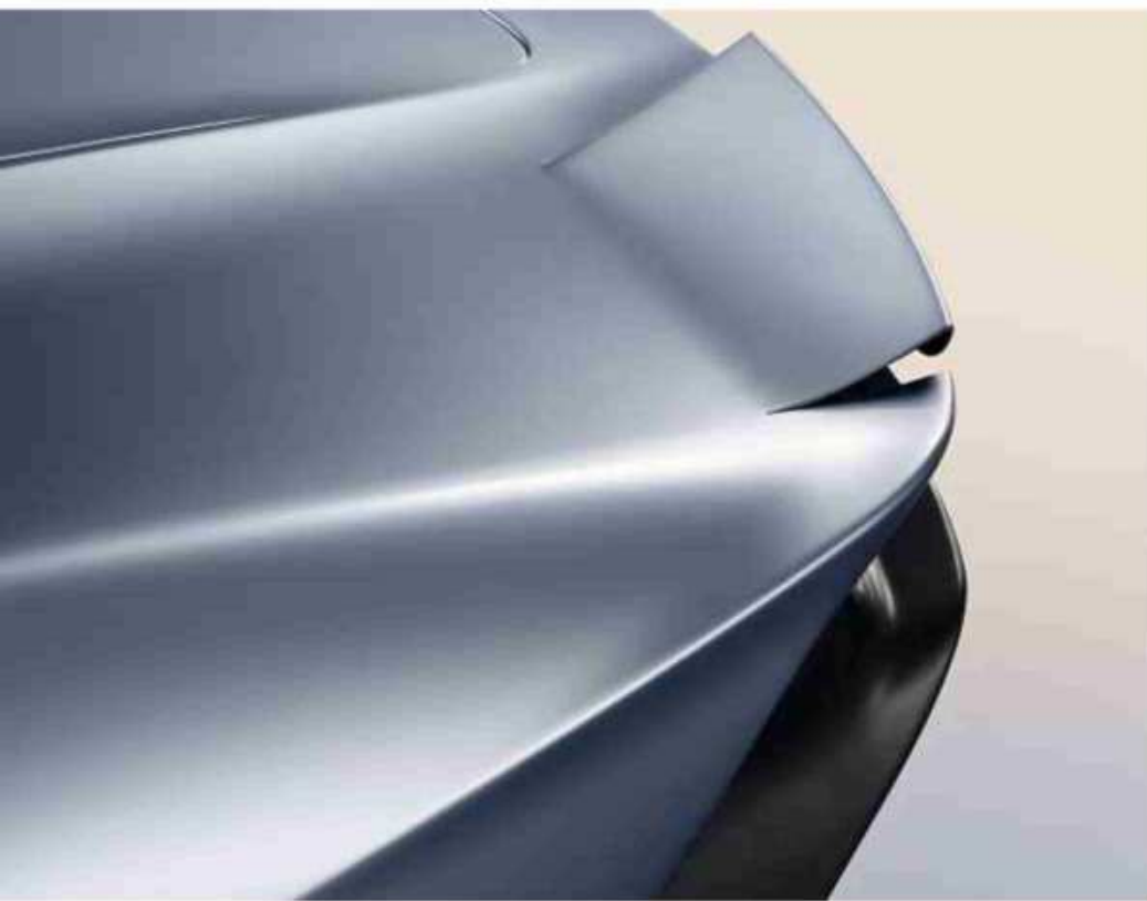
Left: flexible carbon ailerons trim aero as required. Right: front wheel hubs hide carbon brakes shared with the Senna
